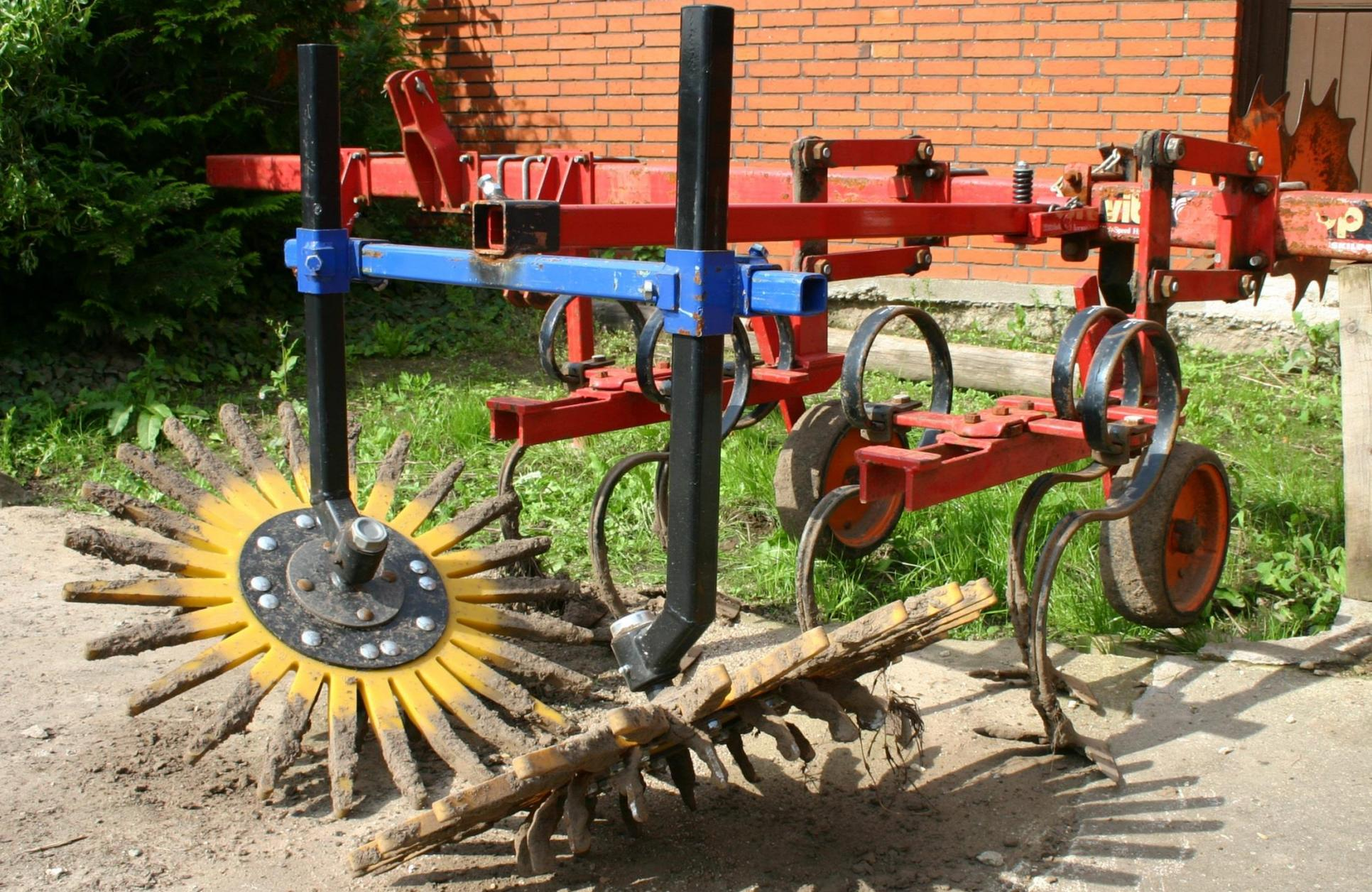
A large red Kress Fingerweeder machine is shown, mounted on a tractor. The machine features a prominent circular head with a yellow and black design, which is used for weeding. The tractor is red and has a blue frame. The machine is parked on a dirt path next to a brick building. The background shows green foliage and a wooden fence.
